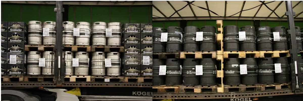
Fig. 1: Sensible arrangement for mixed loads Fig.2: Pallets can help when barrels only are being transported (Formation of "form-locking compartments" using crates for not more than 6 X 6 steel barrels (total 36 barrels per layer) in the loading area)
