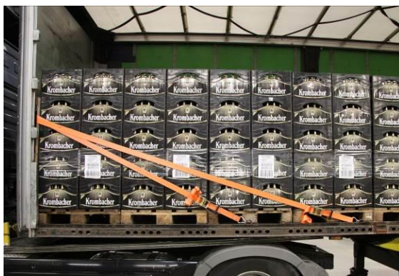
Fig. 3: Securing the front wall
