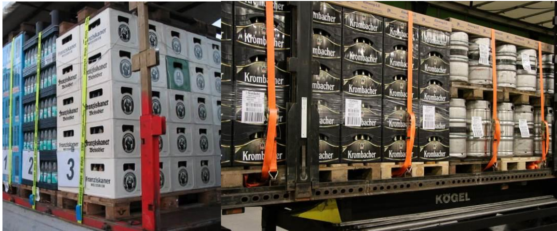
Figs. 4 & 5: Pallets or suitable edge protection angles are required for stabilisation and lashing
